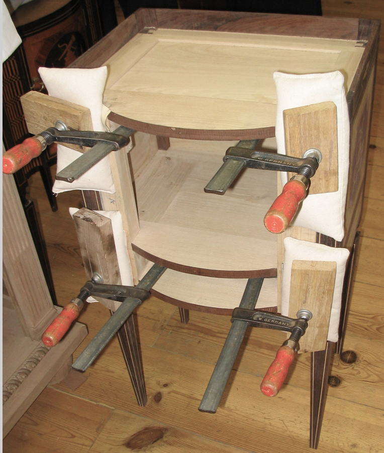
Figure 10.23d Veneer being glued to the surface of a cabinet at the Ricardo do Espirito Santo Silva Foundation, Lisbon, Portugal (photograph by Carol Ventura, 2005).
