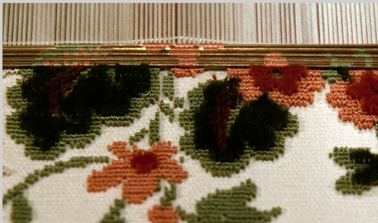
Figure 10.30d Velvet wires on cut and uncut voided velvet fabric on a loom at Rubelli in Como, Italy (photograph by Carol Ventura, 2013).
