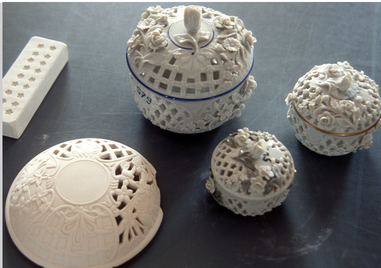
Figure 11.27g Rectangular sprig mold , partially pierced slip-cast porcelain vessel, three finished pierced covered porcelain vessels embellished with press molded and modeled flowers and overglaze in the Dresden Porcelain Factory, Germany (photograph by Carol Ventura, 2009).
