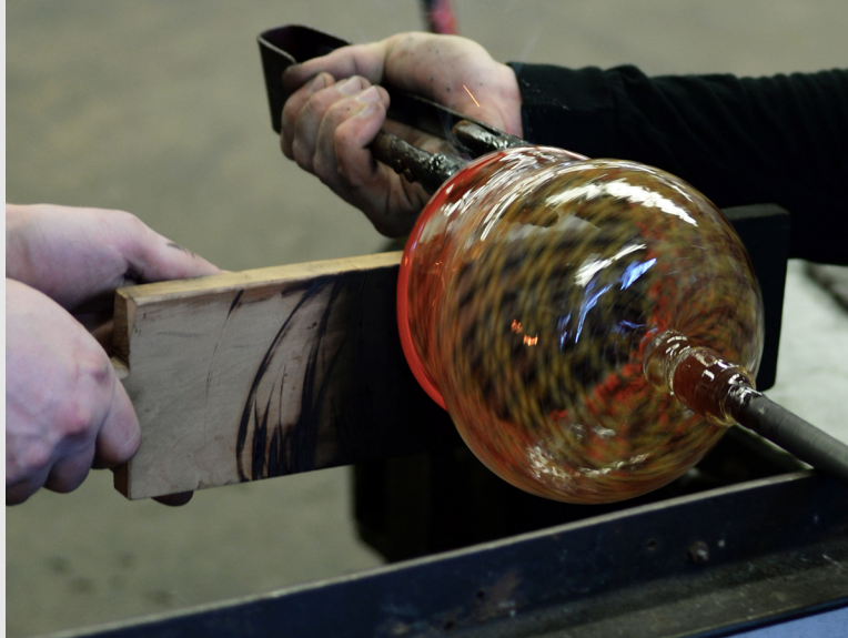
Figure 11.10y The vessel is reheated and opened with jacks while rotating the pipe at the Appalachian Center for Craft in Smithville, TN (photograph by Carol Ventura, 2015).
