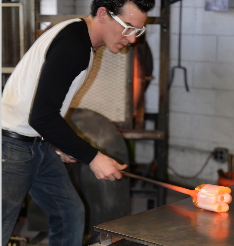
Figure 11.8d John rolls the hot glass on the marver to form it into a cylinder at the Appalachian Center for Craft in Smithville, TN (photograph by Carol Ventura, 2015).
