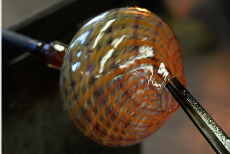
Figure 11.10w The hole in the top of the hot vessel attached to the punty is enlarged with jacks at the Appalachian Center for Craft in Smithville, TN (photograph by Carol Ventura, 2015).
