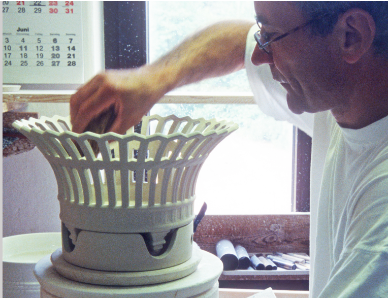
Figure 11.27f Smoothing the surface of the damp porcelain basket with a sponge on a kick wheel in the Dresden Porcelain Factory, Germany (photograph by Carol Ventura, 2009).
