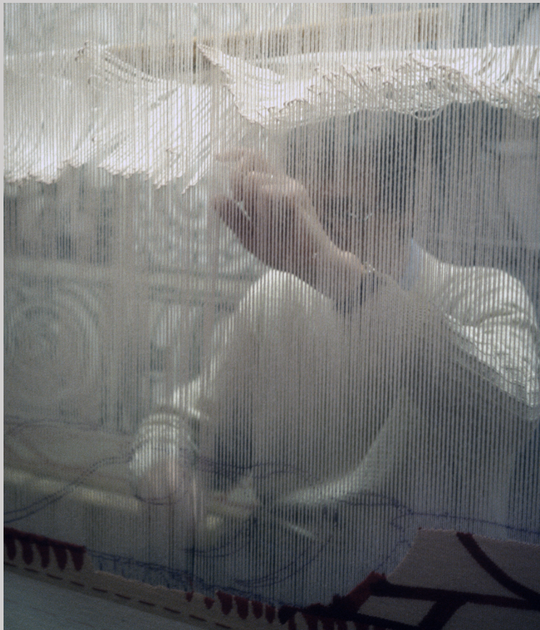
Figure 11.6b Detail of pile warp of a Savonnerie high warp loom at Gobelins Manufactory in Paris, France (photograph by Carol Ventura, 2001).
