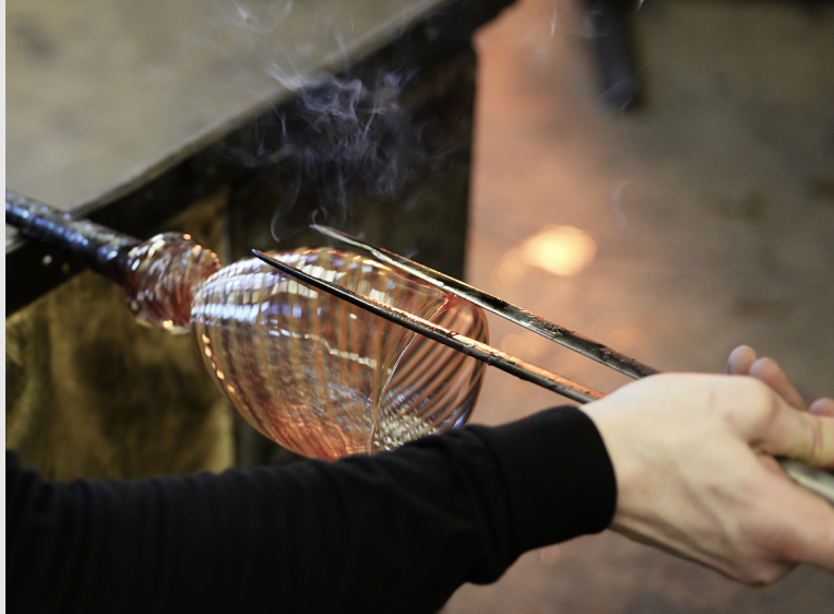
Figure 11.10n The shape is refined with wax-covered jacks as the pipe is rotated at the Appalachian Center for Craft in Smithville, TN (photograph by Carol Ventura, 2015).
