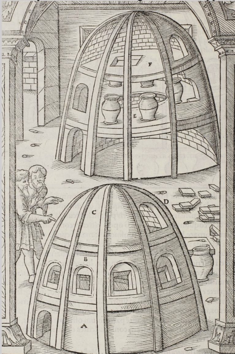
Figure 10.8a Venetian glass furnace, in De re metallica by Georg Agricola (German, 1494–1555) page 484 (The Corning Museum of Glass, Rakow
