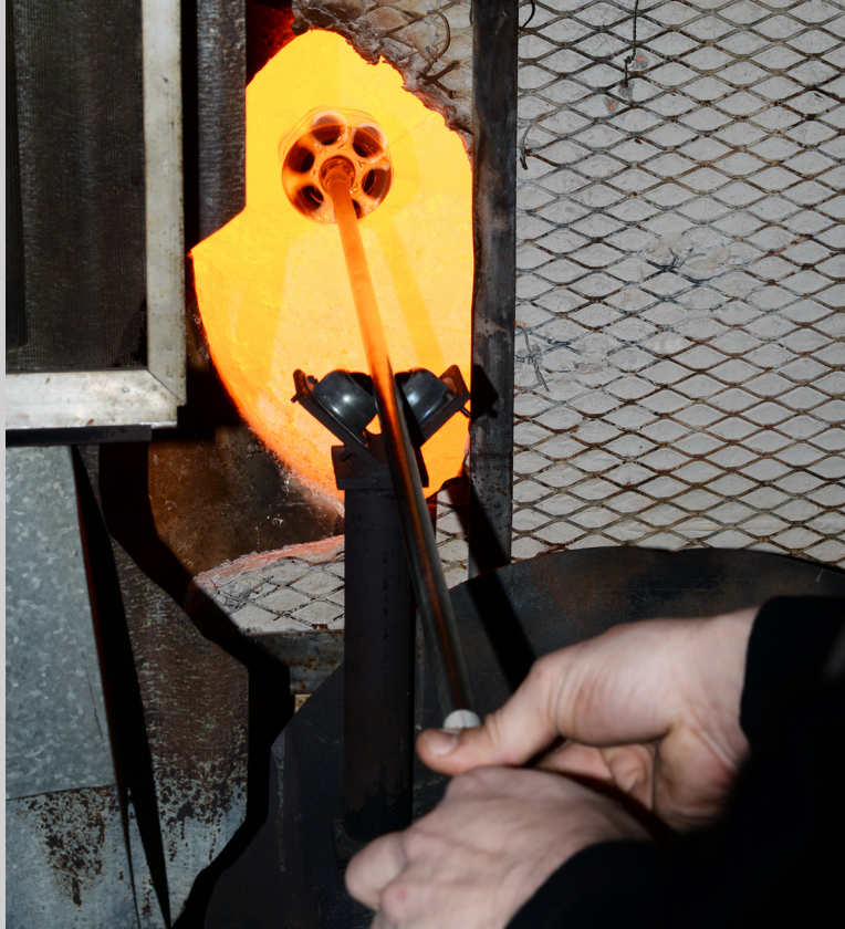
Figure 11.8c The glass bundle is heated in a glory hole at the Appalachian Center for Craft in Smithville, TN (photograph by Carol Ventura, 2015).
