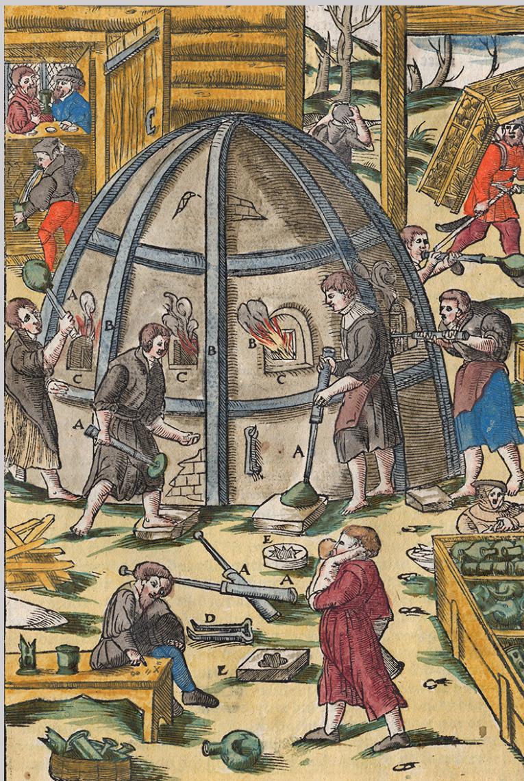
Figure 10.8b Working Venetian glass furnace, in De re metallica by Georg Agricola (German, 1494–1555) page 486 (The Corning Museum of Glass).
