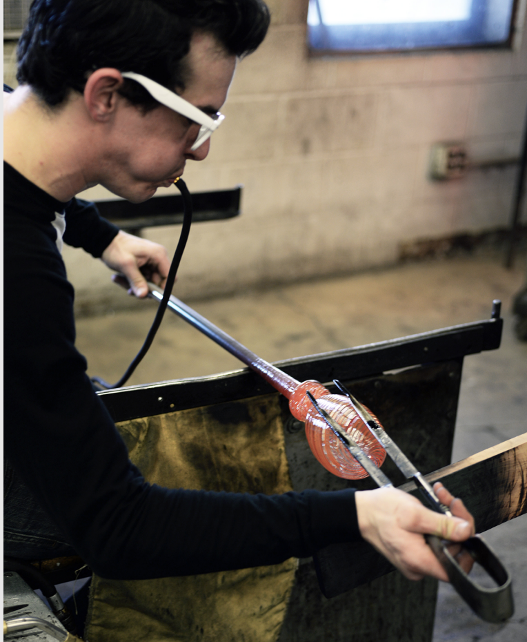
Figure 11.10i John rotates the pipe and blows through a hose connected to the end of the blowpipe to inflate the vessel while shaping it with jacks at the Appalachian Center for Craft in Smithville, TN (photograph by Carol Ventura, 2015).
