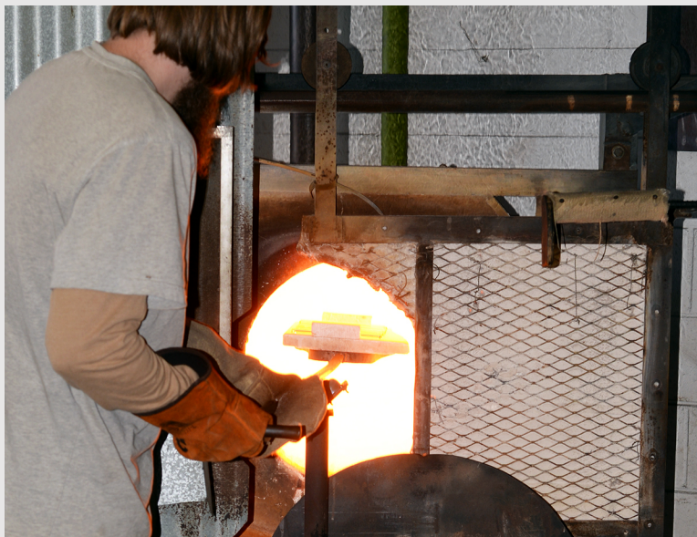
Figure 11.10b The canes on the ferro are fused together in a hot glory hole at the Appalachian Center for Craft in Smithville, TN (photograph by Carol Ventura, 2015).
