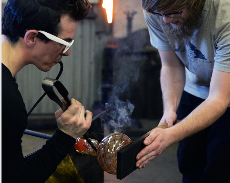
Figure 11.10u The neck is cinched in with jacks as the bottom is flattened with a wood paddle while the pipe is rotated and air is blown into the vessel at the Appalachian Center for Craft in Smithville, TN (photograph by Carol Ventura, 2015).
