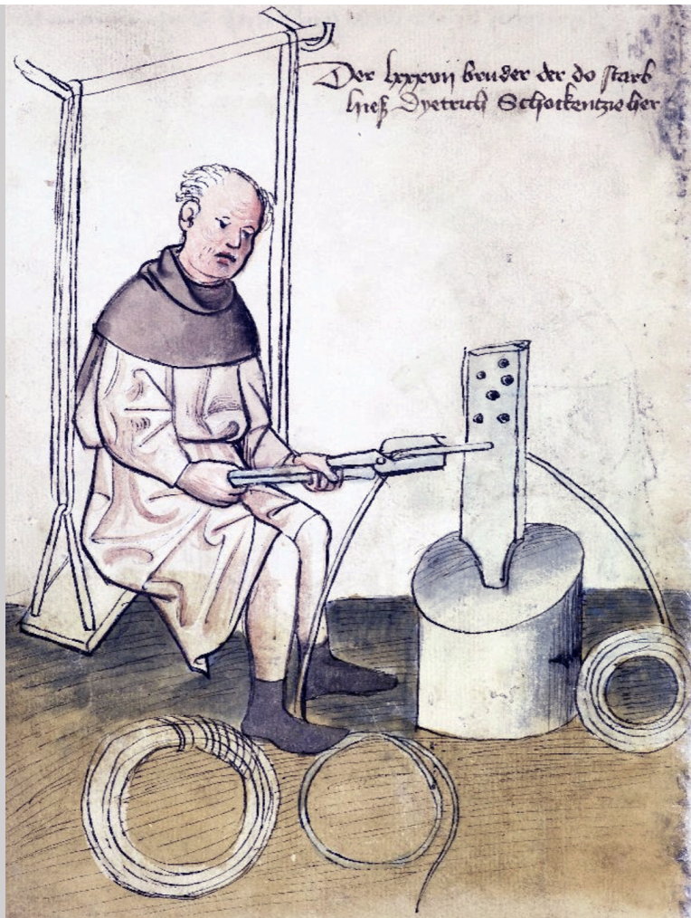
Figure 10.16b Drawing wire through in iron drawplate with draw tongs from Das Hausbuch der Mendelschen Zwolfbruderstiftung by Nurnberg ca. 1425. (Mendel I, Amb. 317.2, Folio 40 verso). https://online-service.nuernberg.de/viewer/image/5d64f831-7a9d-47b4-9a01-d6a28f29ad99/85/LOG_0085/
