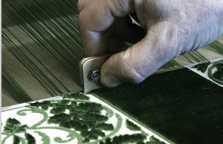
Figure 10.30c Cutting velvet loops on the wire at the Lisio Foundation, Florence, Italy (photograph by Carol Ventura, 2013).
