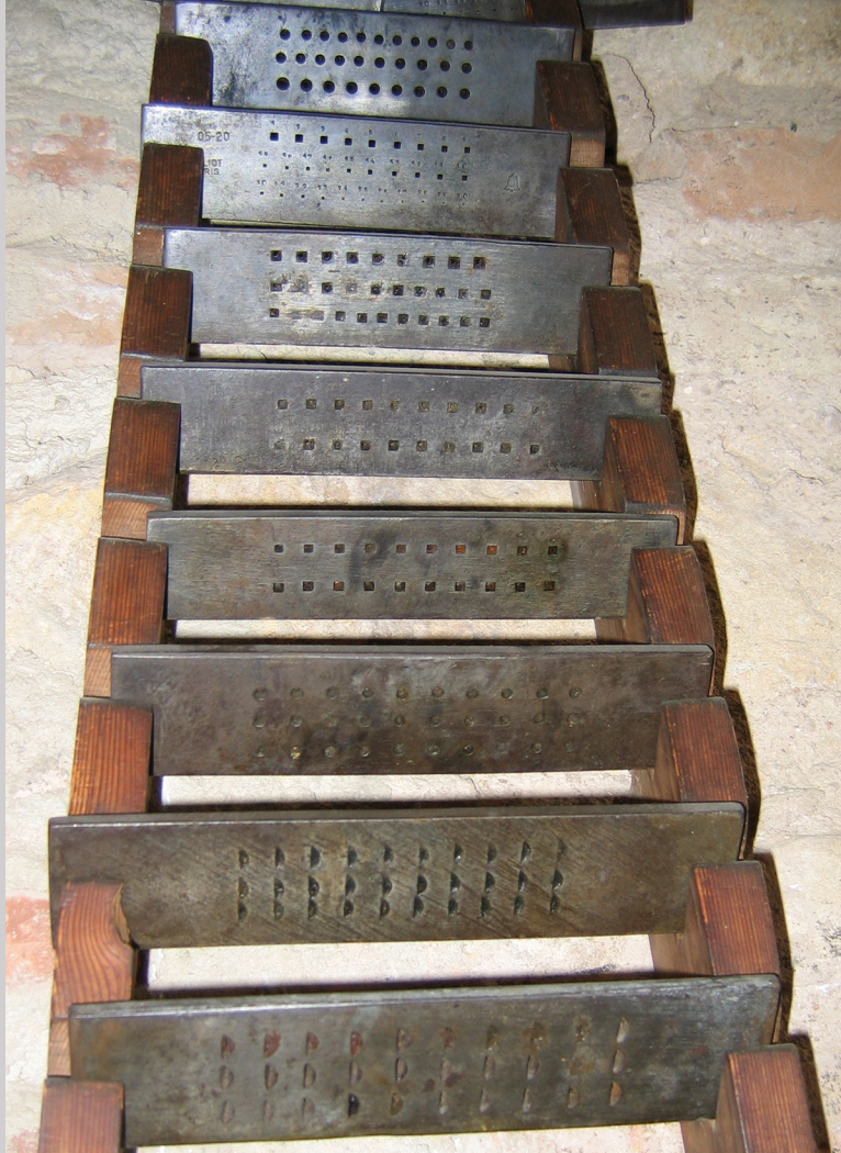
Figure 10.16d Iron drawplates with shaped diminishing sized holes used with the wire puller in Figure 10.16c in the Museo Regina de Joyería, Córdoba, Spain (photographs by Carol Ventura, 2005).
