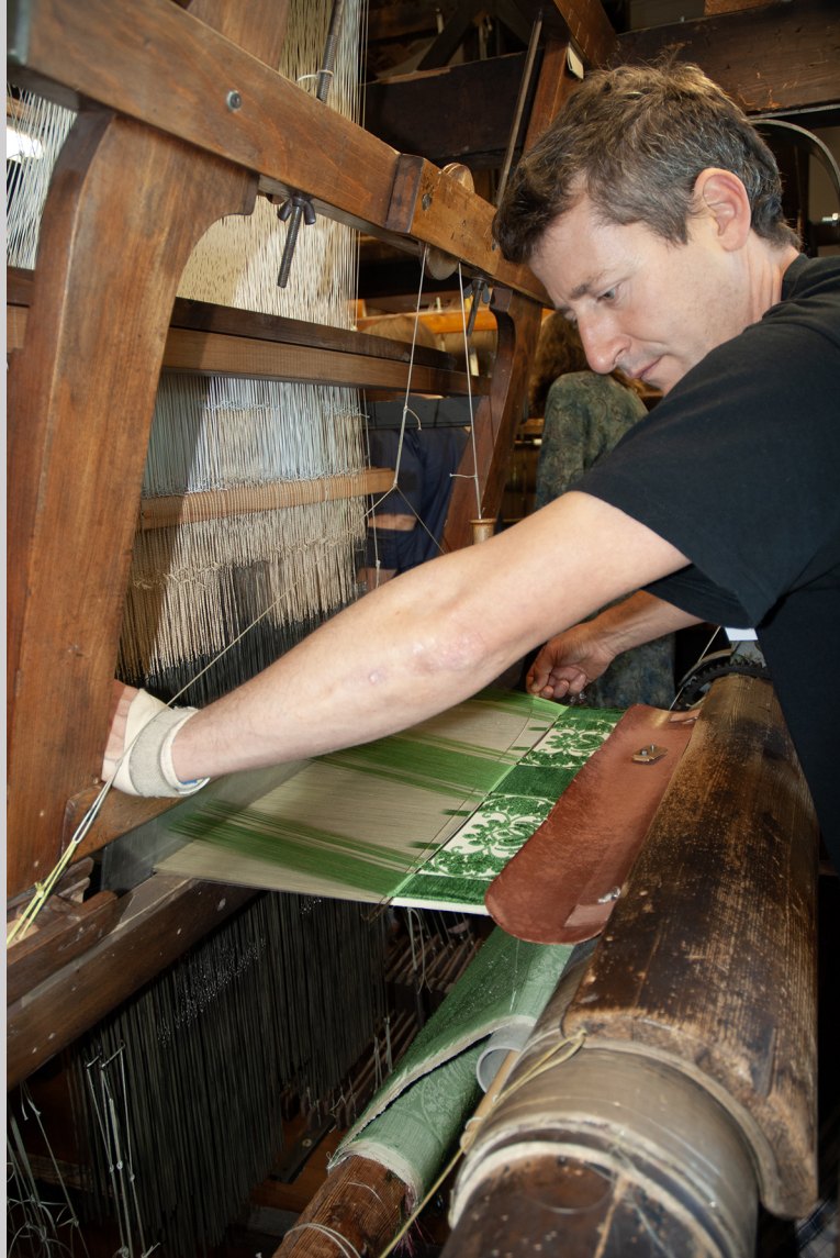
Figure 10.30b Inserting wire into the shed at the Lisio Foundation, Florence, Italy (photograph by Carol Ventura, 2013).
