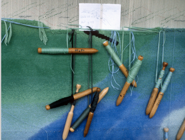
Figure 11.6b Detail of pile warp of a Savonnerie high warp loom at Gobelins Manufactory in Paris, France (photograph by Carol Ventura, 2001).
