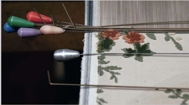
Figure 10.30d Velvet wires on cut and uncut voided velvet fabric on a loom at Rubelli in Como, Italy (photograph by Carol Ventura, 2013).
