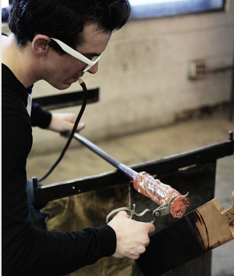
Figure 11.10h John rotates the pipe as he cuts off the top of the vessel with shears while Wes shields John's hand from the heat with a wet wooden paddle at the Appalachian Center for Craft in Smithville, TN (photograph by Carol Ventura, 2015).
