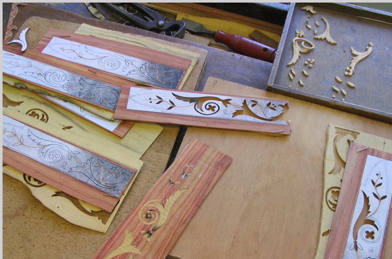
Figure 10.23c A disassembled packet of components being assembled to prepare marquetry panels at the Ricardo do Espirito Santo Silva Foundation, Lisbon, Portugal (photographs by Carol Ventura, 2005).
