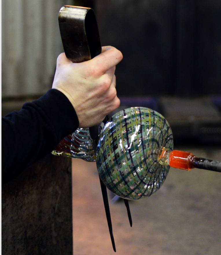
Figure 11.10v The neck is reduced with jacks to ready it for the sculpted punty, which is attached in the middle of the bottom of the double vessel at the Appalachian Center for Craft in Smithville, TN (photograph by Carol Ventura, 2015).
