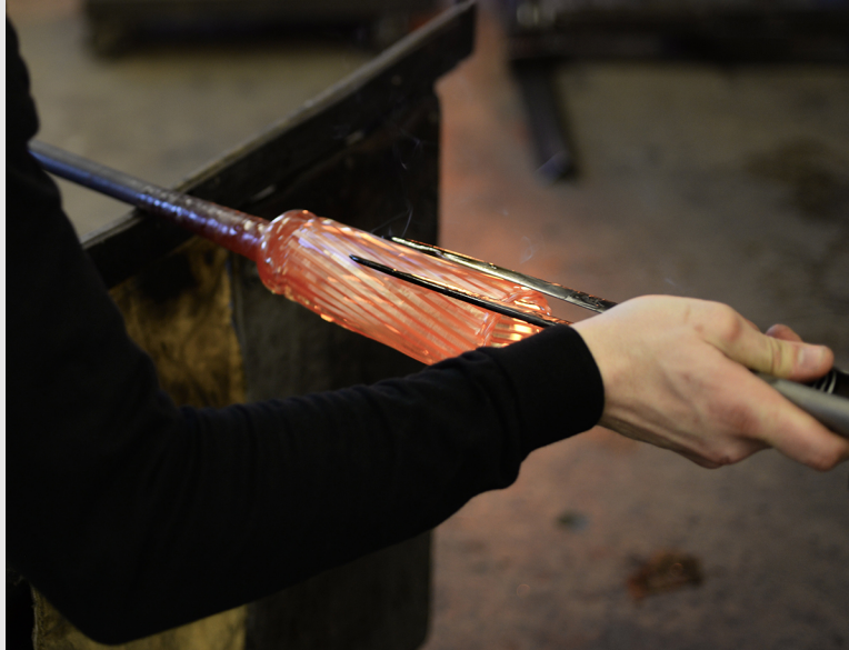
Figure 11.10e John shapes and twists the sides with jacks while rotating the pipe at the Appalachian Center for Craft in Smithville, TN (photograph by Carol Ventura, 2015).
