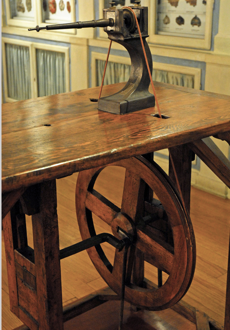
Figure 10.22c Foot-powered grinding wheel to cut into or refine the shape of a stone in the Opificio Pietre Dure Museum, Florence, Italy (photograph by Carol Ventura, 2010).
