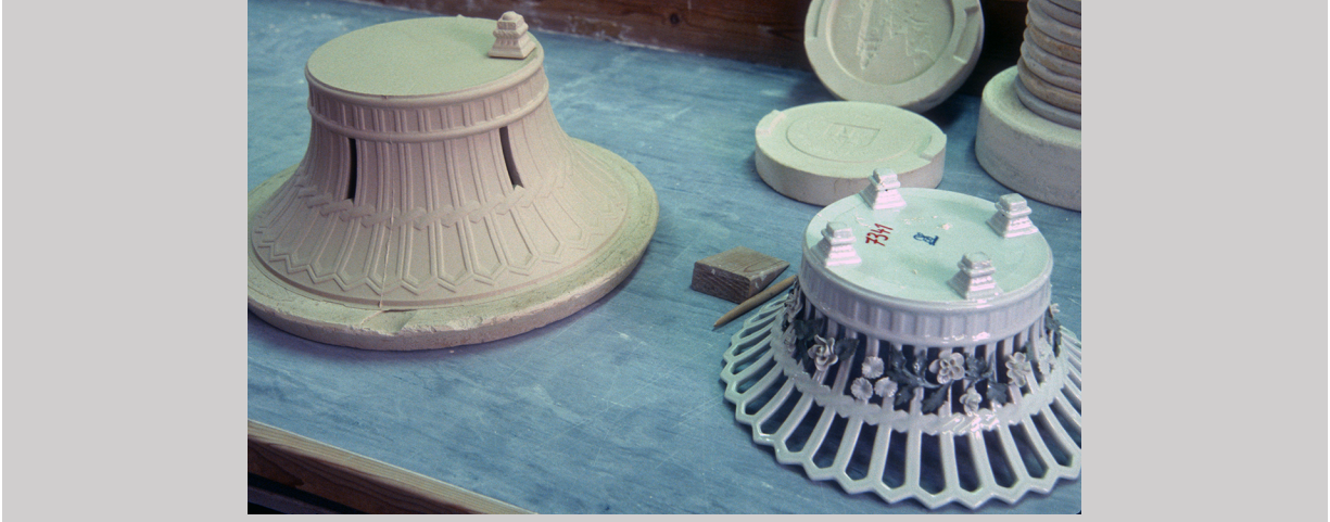
Figure 11.27d Partially pierced damp porcelain basket, upside down finished pierced porcelain basket, and circular two-piece mold in the Dresden Porcelain Factory, Germany (photograph by Carol Ventura, 2009).
