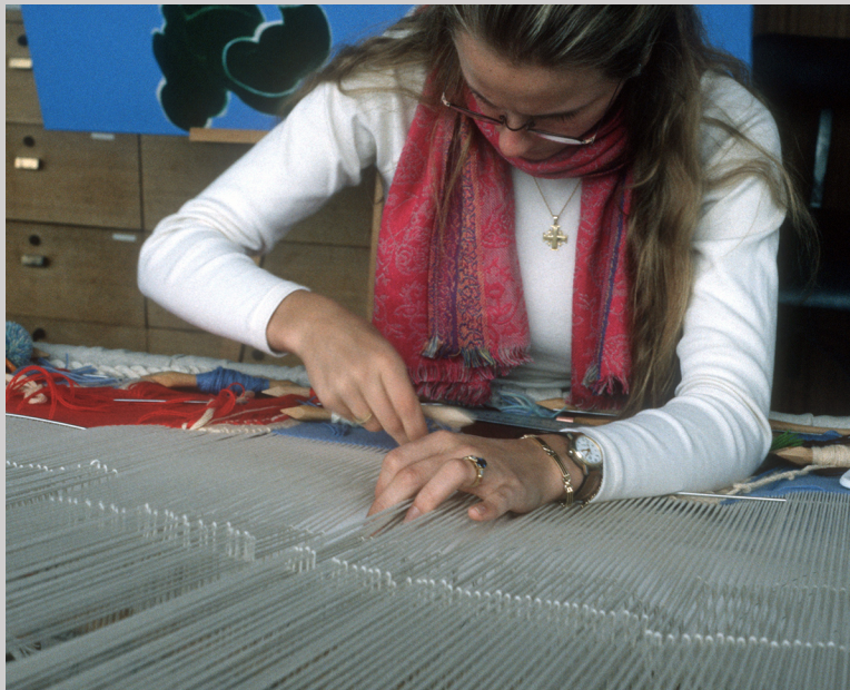
Figure 11.6e Tapestry weaving on Beauvais low warp looms at Gobelins Manufactory in Paris, France (photograph by Carol Ventura, 2001).
