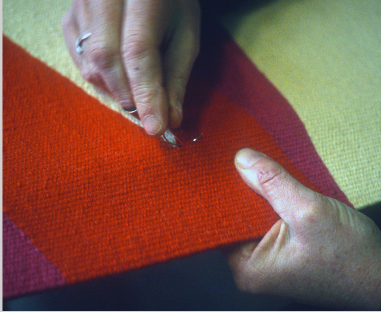
Figure 11.6h Stitching together slits formed between colors with a curved needle and red yarn on a tapestry at Gobelins Manufactory in Paris, France (photograph by Carol Ventura, 2001).
