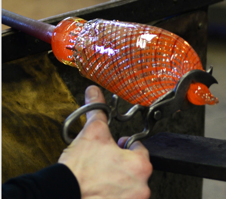
Figure 11.10t Then the knob is sheared off while the pipe is rotated at the Appalachian Center for Craft in Smithville, TN (photograph by Carol Ventura, 2015).
