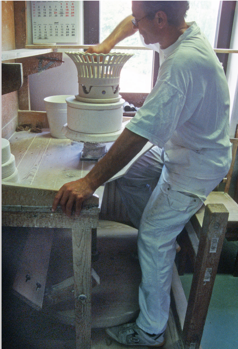
Figure 11.27e Smoothing the damp porcelain basket with a sponge on a kick wheel in the Dresden Porcelain Factory, Germany (photograph by Carol Ventura, 2009).
