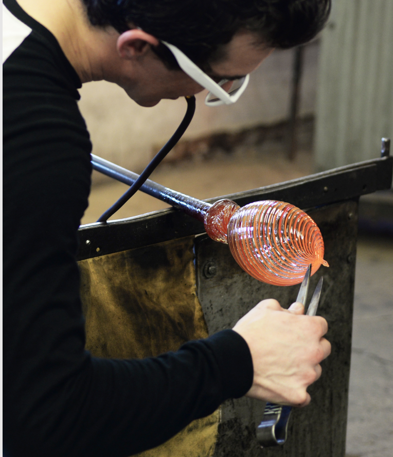
Figure 11.10j John rotates and blows into the pipe while grabbing the tip of the vessel with tweezers at the Appalachian Center for Craft in Smithville, TN (photograph by Carol Ventura, 2015).
