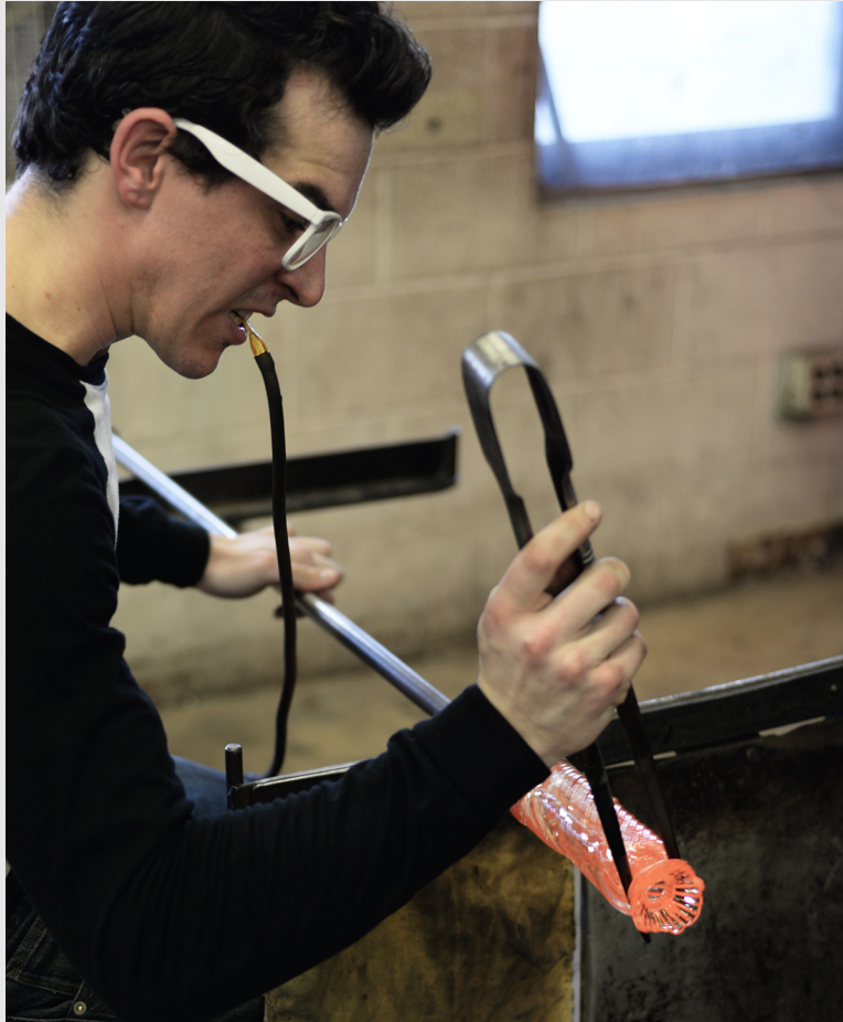
Figure 11.10g John rotates the pipe as he cinches and twists the top of the vessel with jacks at the Appalachian Center for Craft in Smithville, TN (photograph by Carol Ventura, 2015).
