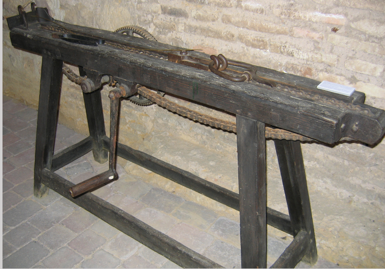
Figure 10.16c Wire puller used with the iron drawplates in Figure 10.16d in the Museo Regina de Joyería, Córdoba, Spain (photographs by Carol Ventura, 2005).
