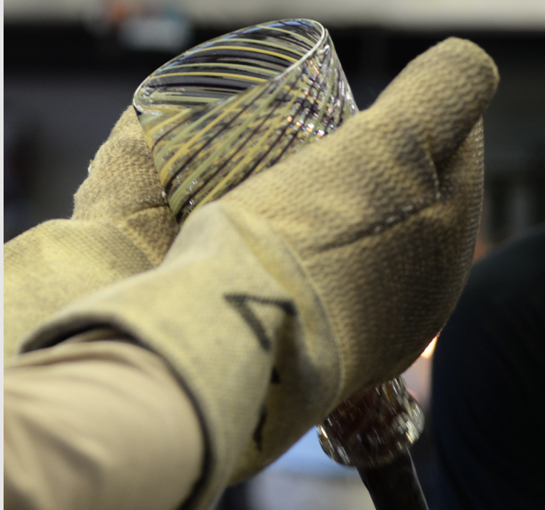
Figure 11.10o The vessel is removed from the pipe and placed in a kiln to keep it hot at the Appalachian Center for Craft in Smithville, TN (photograph by Carol Ventura, 2015).
